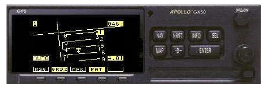
Activate HOLD ASAP (Press GPS SEQ key on panel – OBS Hold light on) (note GX55 hold procedure is different) If not directed to Waypoint 1, activate FPL 0 to 1 leg Press GRD to view grid lines Use small knob to select scale After passing waypoint 0, remove HOLD (Press GPS SEQ key on panel) Press PAT when you desire to abort search pattern
