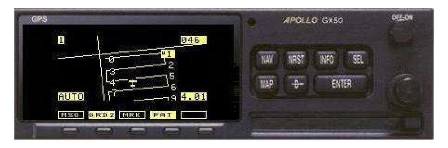
Activate HOLD ASAP (Press GPS SEQ key on panel – OBS Hold light on) (note GX55 hold procedure is different) If not directed to Waypoint 1, activate FPL 0 to 1 leg Use small knob to select scale Press GRD to view grid lines After passing waypoint 0, remove HOLD (Press GPS SEQ key on panel) Press PAT when you desire to abort search pattern
