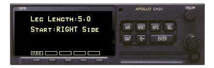
Press SEL Turn SMALL KNOB to bring up next page Press SEL Use Large Knob and small knob to set leg length (0.1 – 9.9 NM) Turn LARGE KNOB to move flashing cursor to Start side Turn SMALL KNOB to select left or right for the first turn
