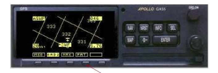
Make sure that SAR mode setup is in place Press MAP to start on Map screen Turn large knob counterclockwise to SAR Map page (has PAT softkey) In the SAR map page press the PAT soft key
