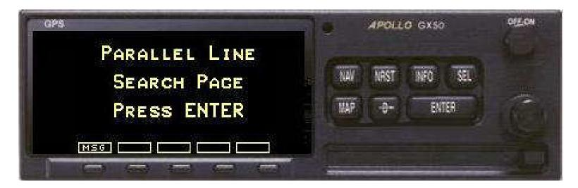
Turn the SMALL KNOB until you see the Parallel Line page Press ENTER to grid setup
