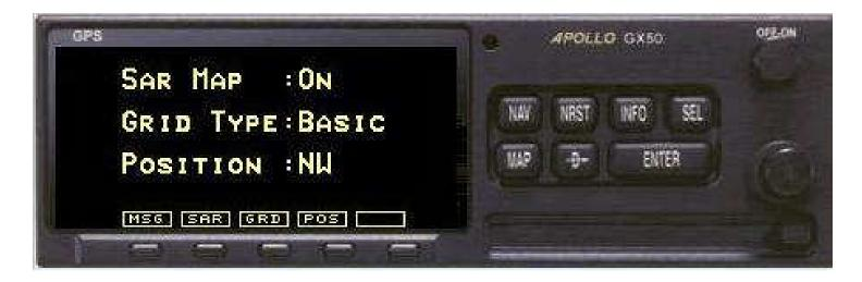
For Parallel Searches using Cell or LAT/LONG set GRID TYPE to BASIC and POSITION to NW which covers all of the US
