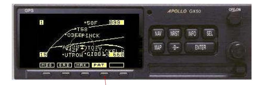
Make sure that SAR mode setup is in place Press MAP to start on the Map screen Turn large knob counterclockwise to SAR Map page (has PAT softkey on the bottom) Press the pattern soft key (PAT)
