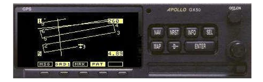
Activate HOLD ASAP (Press GPS SEQ key on panel – OBS Hold light on) (note GX55 hold procedure is different) If not directed to Waypoint 1, activate FPL 0 to 1 leg Use small knob to select scale Press GRD to view Grid Lines After passing waypoint 0, remove HOLD (GPS SEQ key on panel) Press PAT when you desire to abort search pattern
